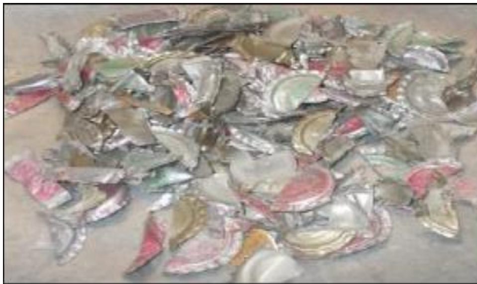
Figure 2. 1. Bottle caps as fibers
