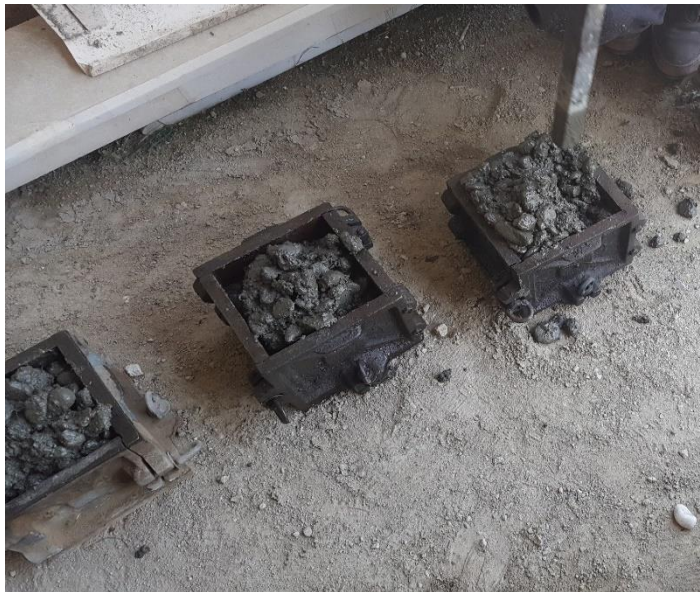
Figure 2. Compaction of the concrete in the cubes
